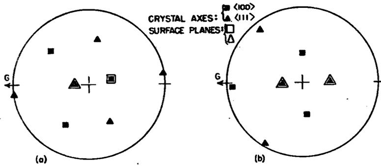
FIG. 2. Stereographic projections of two crystals, showing crystal axes obtained by X-ray diffraction (solid points) and axes of surface planes producing optical reflections (open points). Arrow at G shows growth direction.
