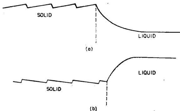
FIG. 1. Advancing interface with surface steps forming (not to scale).
