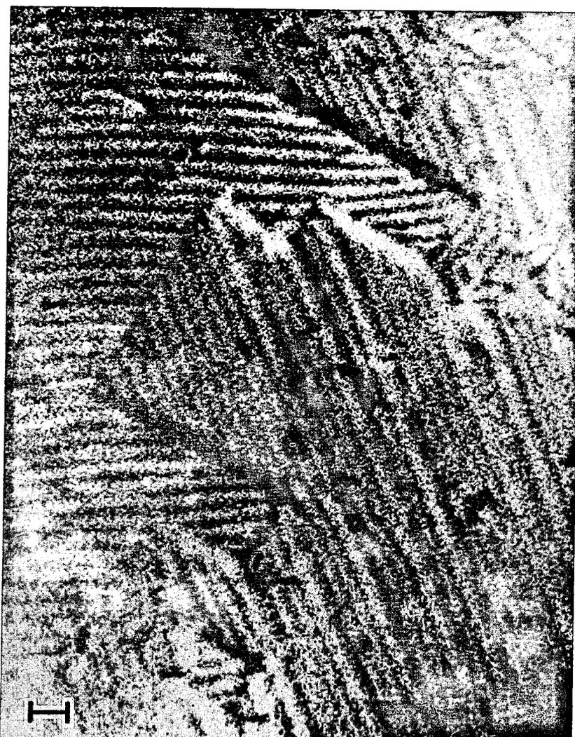
Fig. 2. Magnetic domains in Fe+3.5% Si alloy. Scale mark 25  $\mu$ .
