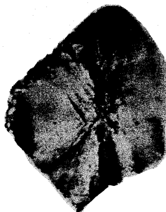
FIG. 5. Section topograph with incident beam cutting crystal along line 5, Fig. 1(c), twin plane reflection.
