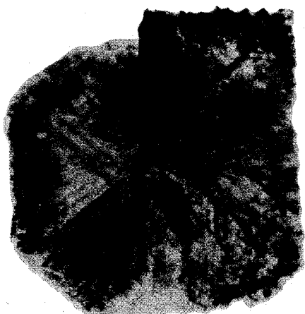
FIG. 3. Projection topograph of major component of twin, reflection from planes parallel to o in Fig. 1(c).
