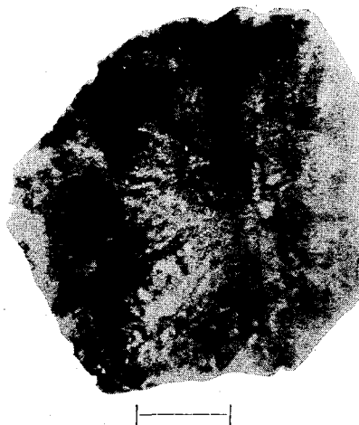
FIG. 2. Projection topograph of synthetic diamond twin, twin plane reflection. Compare shape with Fig. 1(d). Scale mark 100\ \mu .
