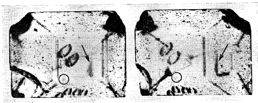
Stereopair of projection topographs, Mo K \alpha radiation. Crystal width is 4 mm. Interior tetrahedron circled, imperfect layer parallel to (111) arrowed. (a) 2\bar{2}0 reflection, (b) 220 reflection.
