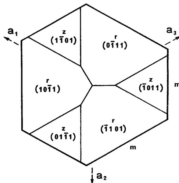
FIG. 3. Idealized section of a quartz crystal cut parallel to the basal plane showing division into major and minor rhombohedral growth sectors. Traces of  $r$ - $z$  growth sector boundaries are parallel to  $\{10\bar{1}0\}$  and  $r$ - $r$  to  $\{1120\}$ . Growth layers parallel to  $r$  and  $z$  faces would outcrop with traces parallel to the sides of the hexagon, i.e. to  $\{10\bar{1}0\}$ .
