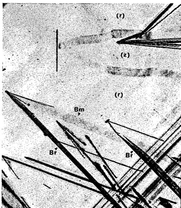
FIG. 2. Topograph of natural quartz plate inclined  $11^\circ$  to major rhombohedron  $(10\bar{1}1)$ . Thickness 1 mm. Reflection  $10\bar{1}\bar{1}$ ,  $\text{AgK}\alpha$  radiation. Field area  $1 \times 1.3$  mm. Marked features explained in text. Plate is viewed along a direction tilted  $40^\circ$  away from the  $c$ -axis towards the normal to  $(10\bar{1}1)$ . Projection of diffraction vector is horizontal, direction  $[\bar{1}2\bar{1}0]$  is vertical on the topograph.
