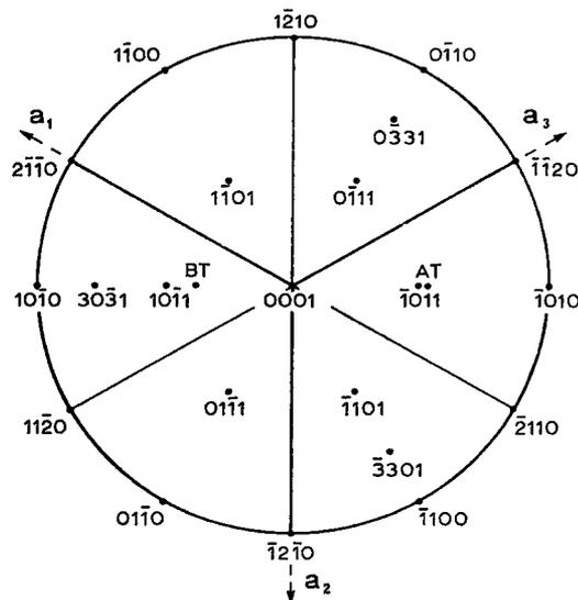
FIG. 1. Stereographic projection parallel to the  $c$ -axis showing poles of the chief planes used in X-ray topographic surveys. The two-fold axes are parallel to the  $a$ -axes and pierce the structure at heights which depend upon the hand of the structure.
