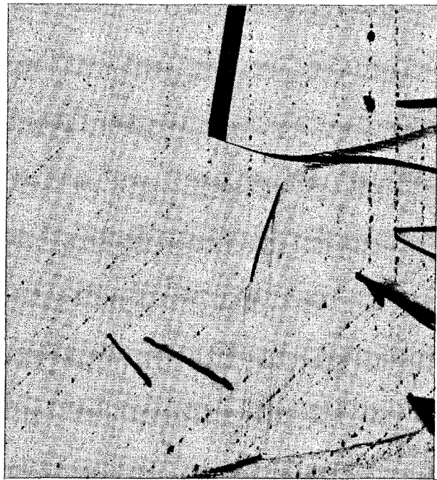
Figure 3. X-ray topograph of natural quartz plate about 1 mm thick. Field edge length 8 mm; reflection 2420, diffraction vector vertical; Mo K_{\alpha} radiation; fault fringes at Dauphiné twin boundaries.
