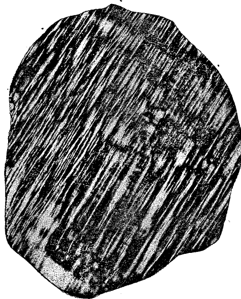
Fig. 3. Birefringence topograph: "tatami" structure. Specimen width 8 mm, thickness 1 mm.
