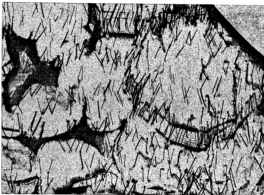
FIG. 5. Topograph of slice cut parallel to (0001) containing part of final growth surface. Thickness 0.7 mm, field width 7 mm. Rhombohedral plane reflection, projections of g and of c axis are vertical. Dislocations and fault surfaces make fairly small angles with [0001].
