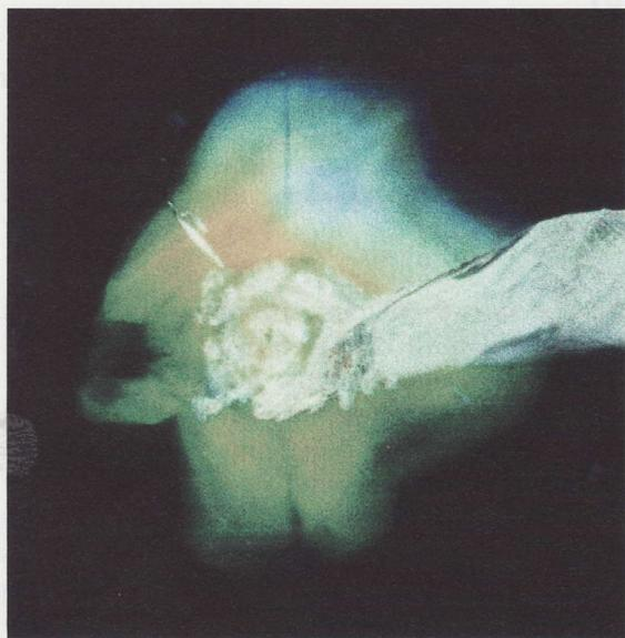
Fig. 6. Colour micrograph of core PL, 325nm excitation, recorded on Kodak Gold 200.
