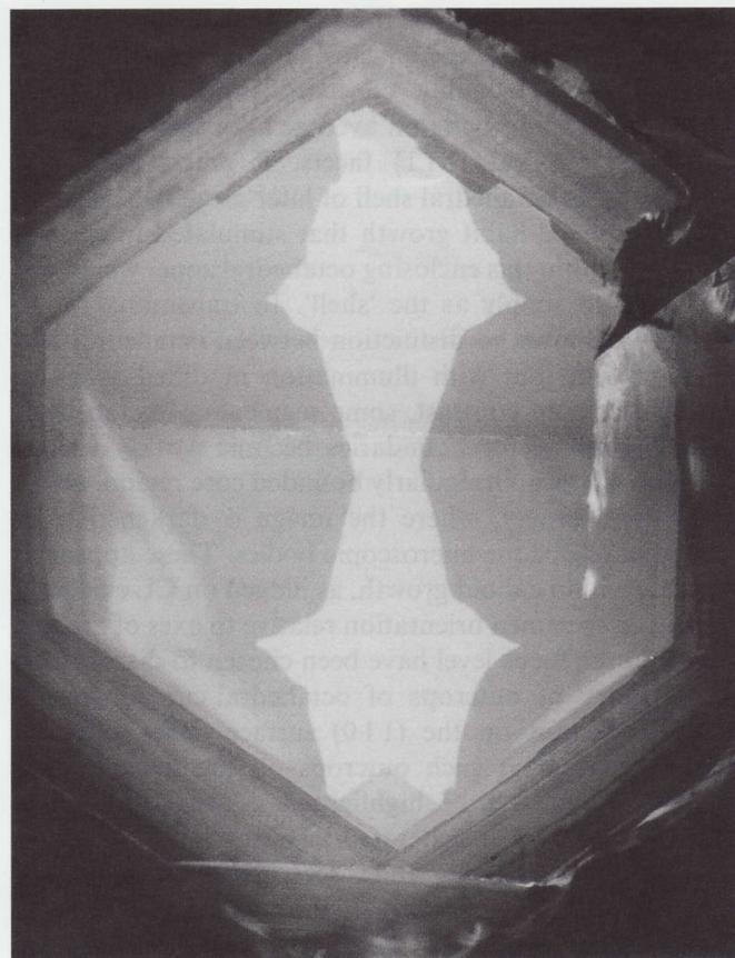
Fig. 4. CL topograph of  $(\bar{1}\bar{1}0)$  surface. Spliced monochrome prints from colour originals, inverted left-to-right so that orientation of  $(\bar{1}\bar{1}0)$  surface appears as if viewed vertically under Fig. 3(a). Electron beam conditions as in Fig. 3. Field width 1.8 mm.
